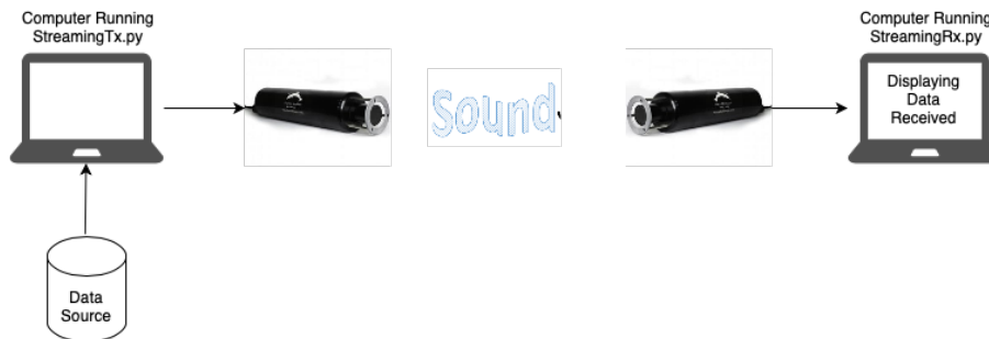
Figure 1.1: Streaming Data setup with 2 Popoto Modems and 2 laptops. The modems are connected via ethernet.
