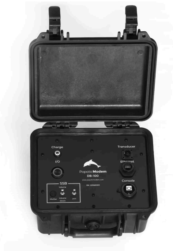
Figure 4.1: The Popoto DB100 Deckbox
