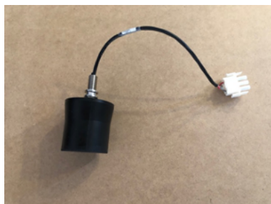
Figure 1.1: The Popoto 25 Khz Transducer
